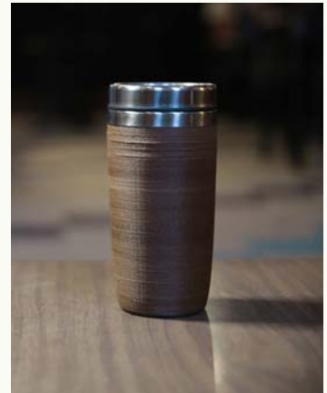
C2cup made of coffee-based biocomposite
